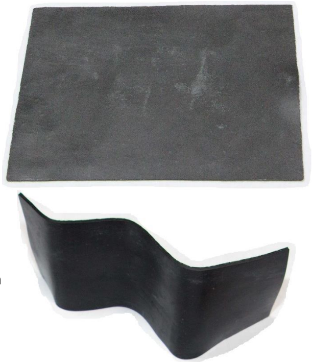
FlexPCC shown as flat sheet and with multiple bends
